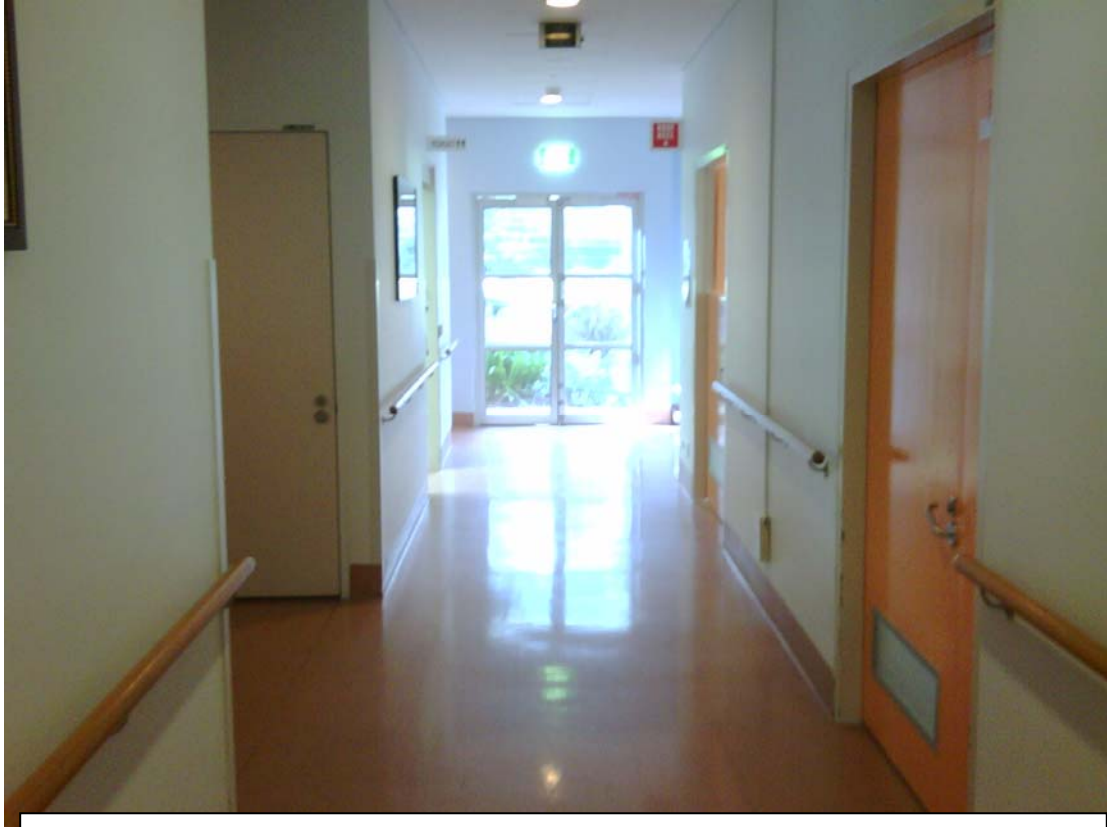
Be aware of the glare reflected off shiny, buffed floor surfaces. Residents can perceive this as a pool of water to be walked around – or waded through. (Brawley)
